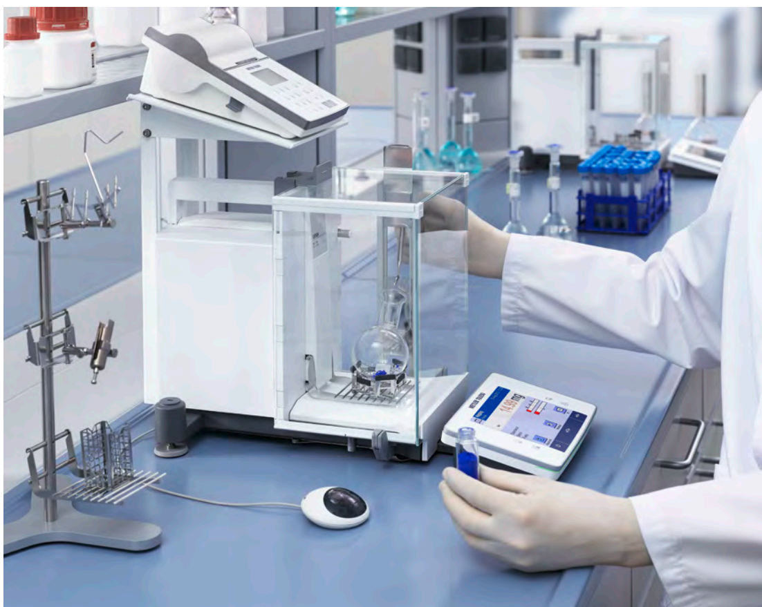
Figure 6: Operate the balance without touching it: Add an optical hand-sensor, configured to open the draft shield door, to tare or to print results simply with a wave of your hand.
