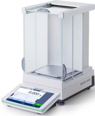
Figure 15: Precision balance with standard weighing pan and draft shield (1 mg readability, XPR1203S) – used in Tests 3(a) and 4(a)
