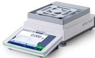
Figure 16: Precision balance with SmartPan Pro (1 mg readability, XPR1203SN) – used in Test 3(b)
