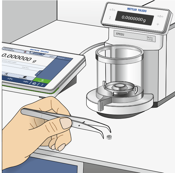
Figure 7: Sample sizes, flasks or crucibles are tiny. Using the appropriate tools will have a positive influence on your weighing in terms of speed, accuracy and convenience.
